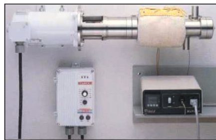
FIGURE 3. Small-scale benchtop evaporators, such as this one, have several advantages (as well as some limitations) for testing and scaleup
