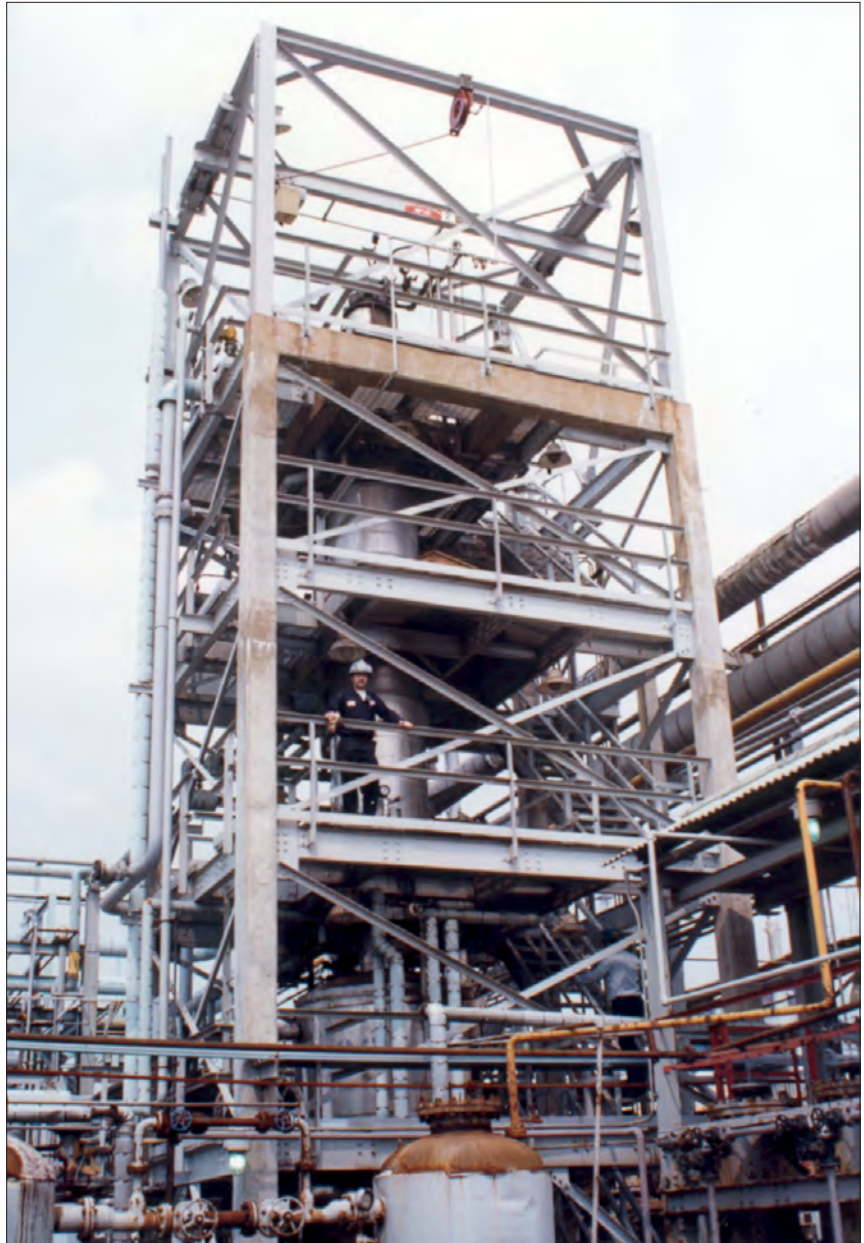
Vistran systems incorporate a special transported thin-film processor which aids the flow of viscous materials.
