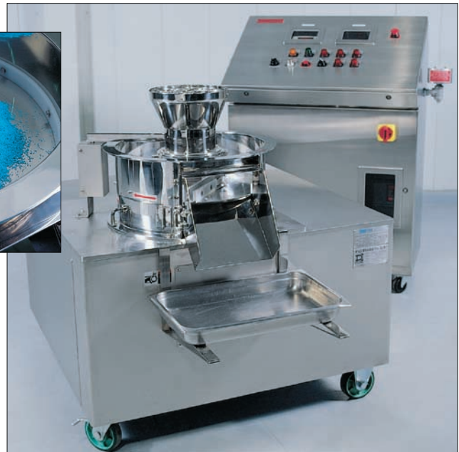
The LCI Basket Granulator is the lowest pressure extruder available
