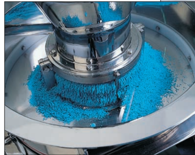
The LCI Basket Granulator is the lowest pressure extruder available
