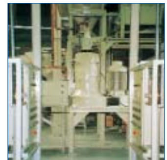
▲ PUR foam conditioning plant for the recycling.
