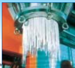
▲ Press 24-390 with overhead drive for pelleting pasty products
