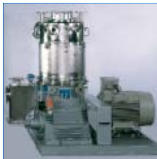
▲ Pelleting press for a chemical product
