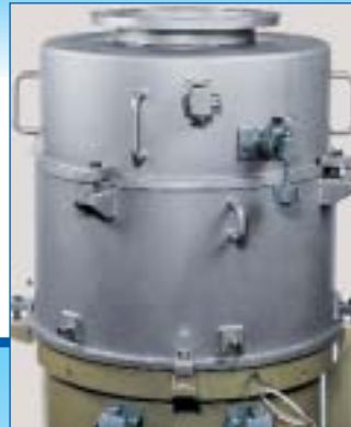
▼ Cooled press cases for thermosensitive products.
