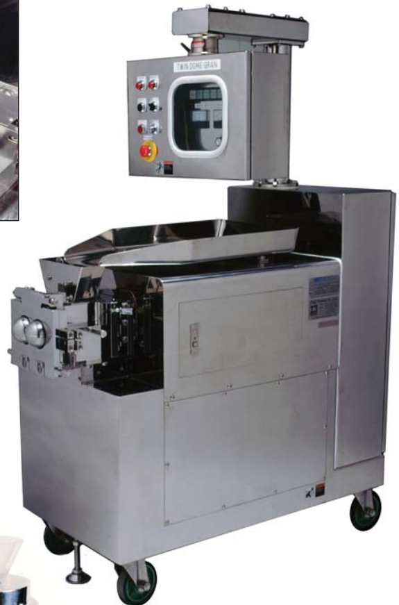
The dome extruder's hemispherical shaped dies result in evenly distributed extrusion forces.
