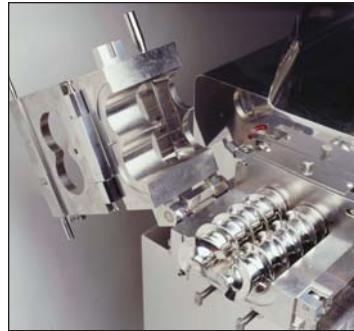
The Twin Dome Granulator's clam shell design allows quick, easy cleaning of the extrusion chamber.
