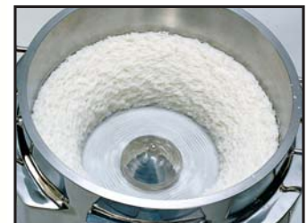
Spheronization produces a smooth particle surface suitable for thin layer coating
