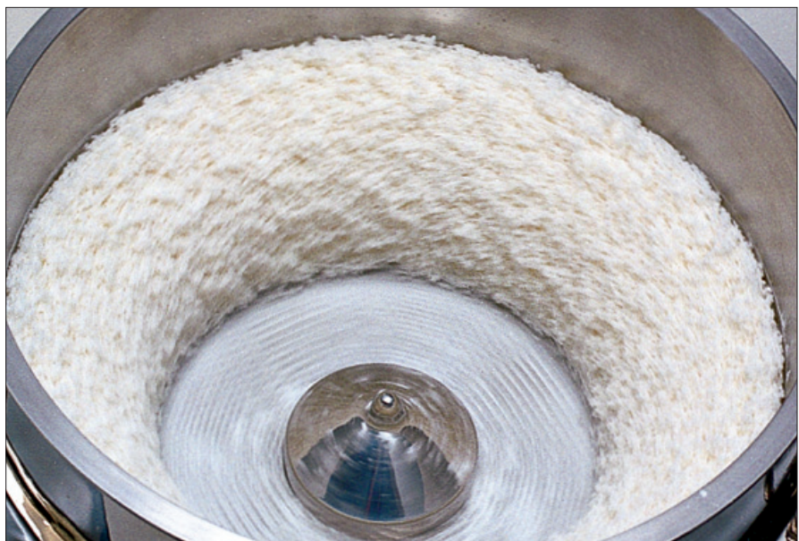
Below: Formation of the spheronizer's "twisting rope".
