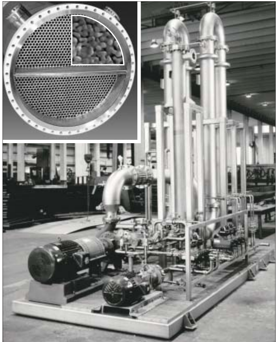
Above: Scepter system. Top left: Scepter filter modules are composed of porous stainless steel tubes with a patented, permanent TiO 2 coating sintered to the tube's inner surface. Inset shows magnified surface of tube coating at 20,000X.
