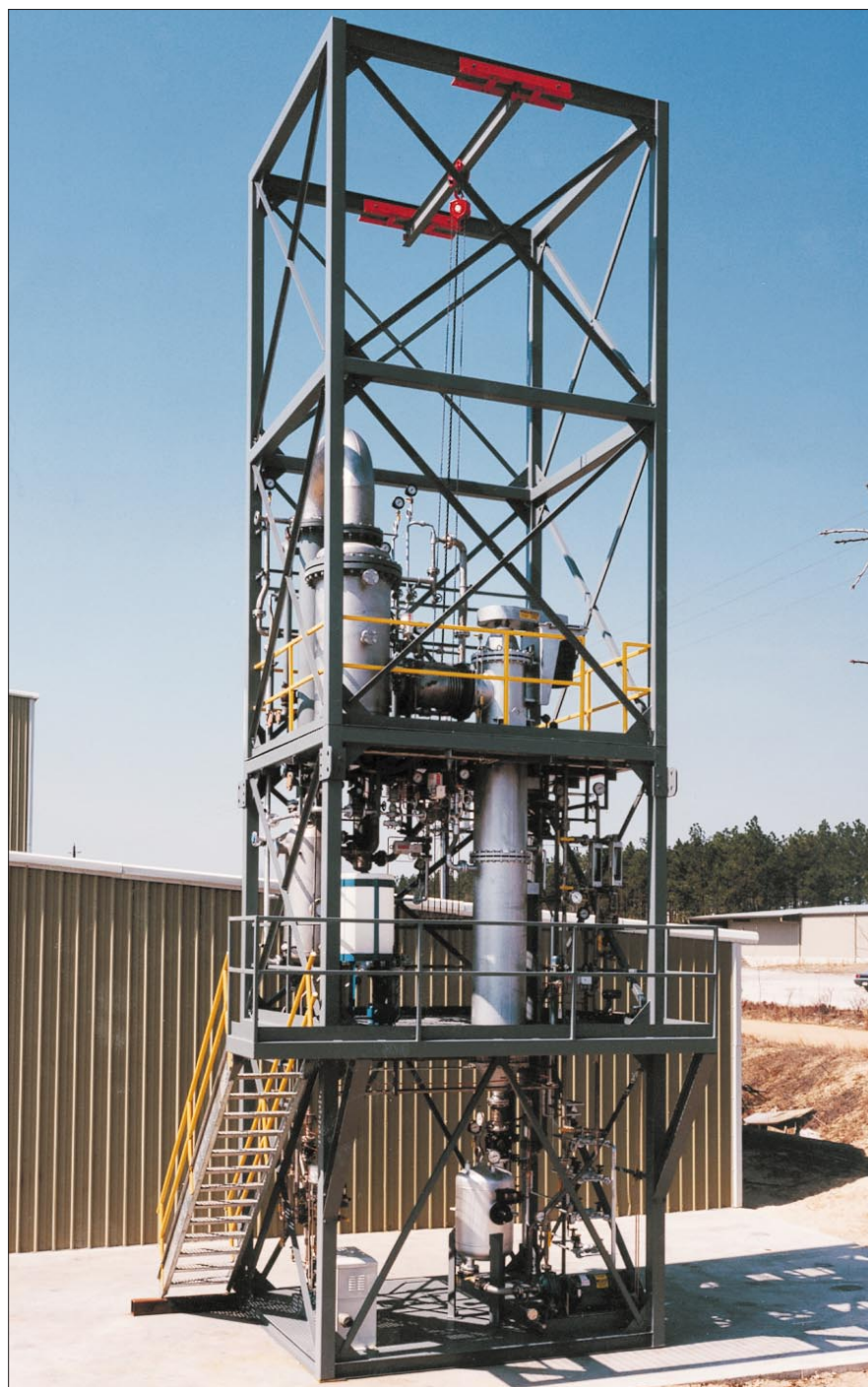
One of a series of LCI custom solvent recovery systems assembled before shipment.
